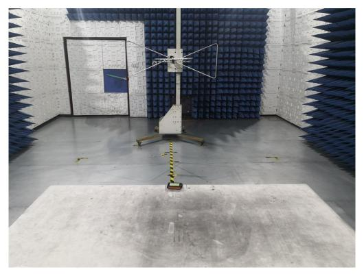
RADIATED EMISSION TEST SETUP ABOVE 1GHZ
