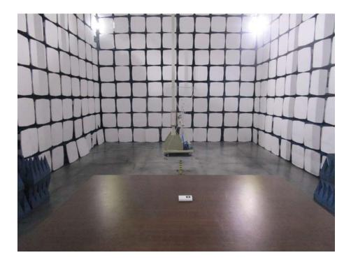
Radiation Emission Test Setup (Above 1GHz)
