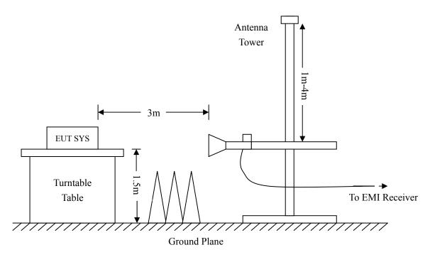
Frequency:9kHz-30MHz Frequency: Above 1GHz Frequency:30MHz-1GHz RBW=10KHz, RBW=120KHz, RBW=1MHz, VBW = 30KHzVBW=300KHz VBW=3MHz(Peak), 10Hz(AV) Sweep time= Auto Sweep time= Auto Sweep time= Auto Trace = max hold Trace = max holdTrace =  $\max$  hold Detector function = peak Detector function = peak, QP Detector function = peak, AV
