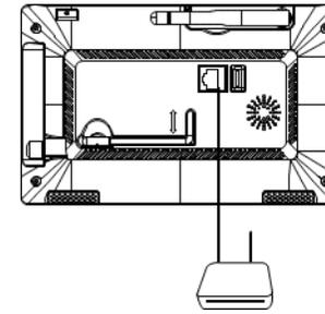
Connect the Monitor to the router by Ethernet cable
