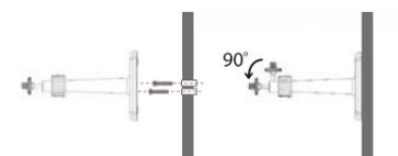
(2) Mount the camera into camera stand. Adjust the viewing angle and fix the camera tightly.
