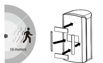
For maximum coverage, it is recommended to place the motion sensor high up with its back against the corner of walls to ensure best detection coverage.
