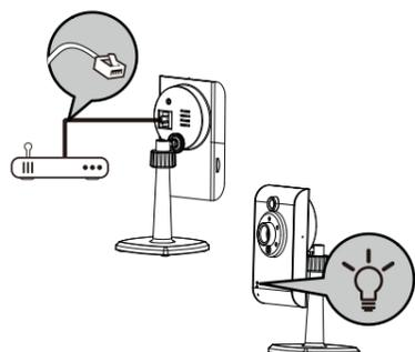
(2) Plug in the power adapter and wait until both RED and GREEN LED begin flashing.
