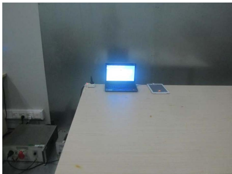
**Radiation Emission Test Setup (9 kHz to 30MHz)**
