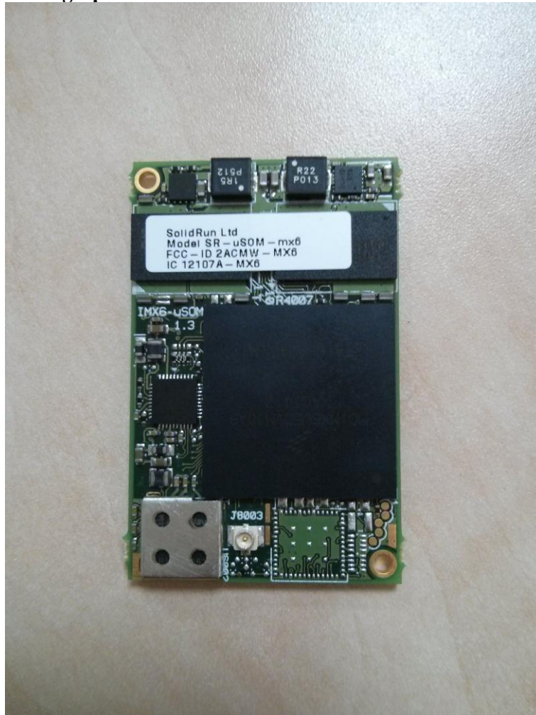
Photograph 1: EUT Side 1- with metal shield on RF section
