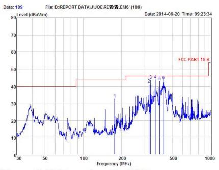
Condition : FCC PART 15 B 3m FOL: HORIZONTAL EUT : Condeco 10.1'' Touch Screen Model No : PN41827
