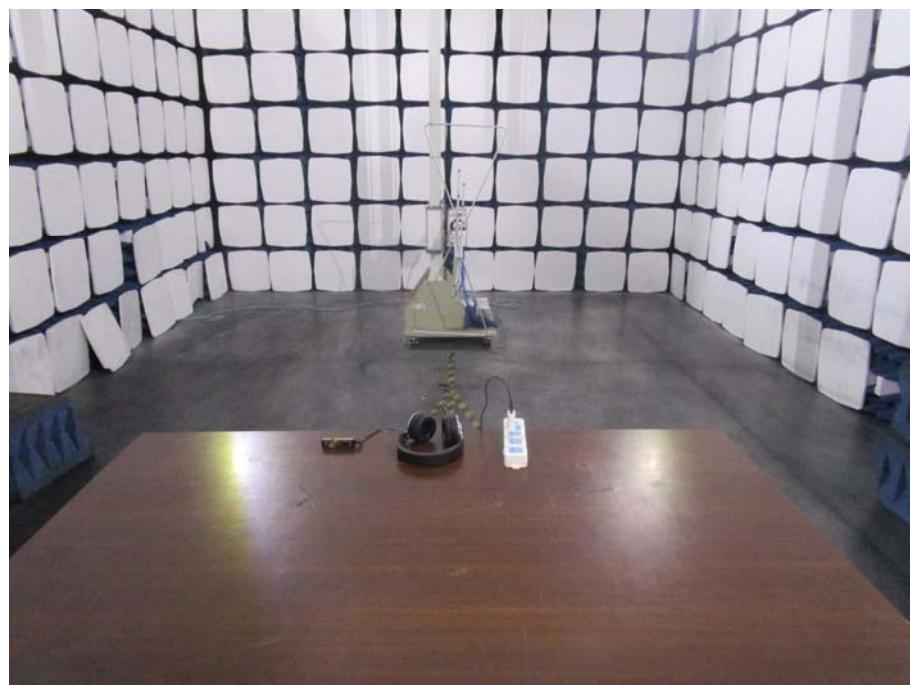
**Radiation Emission Test Setup (Below 30MHz)**
