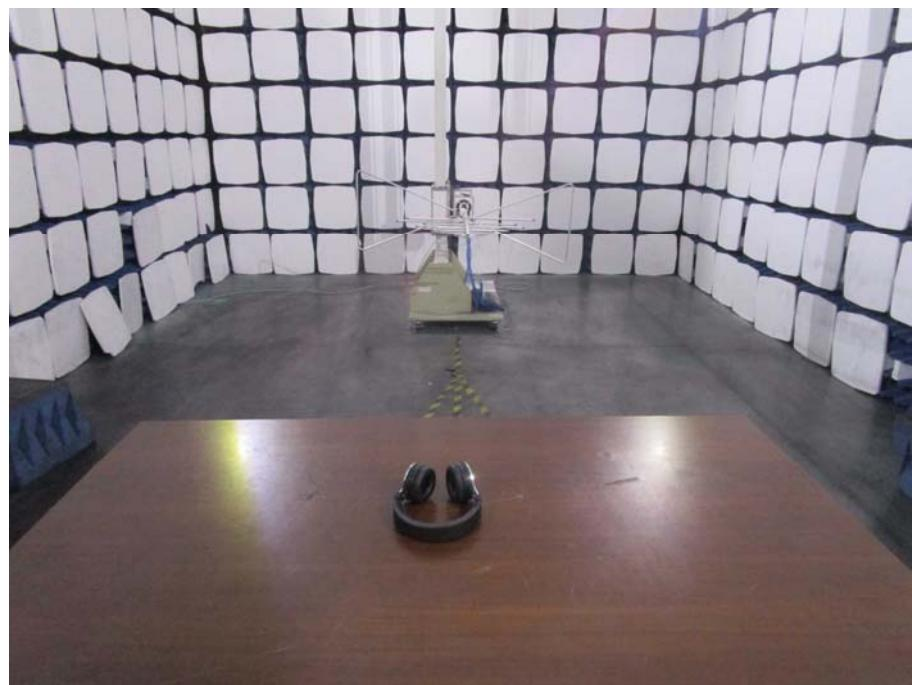
**Radiation Emission Test Setup (Above 1GHz)**
