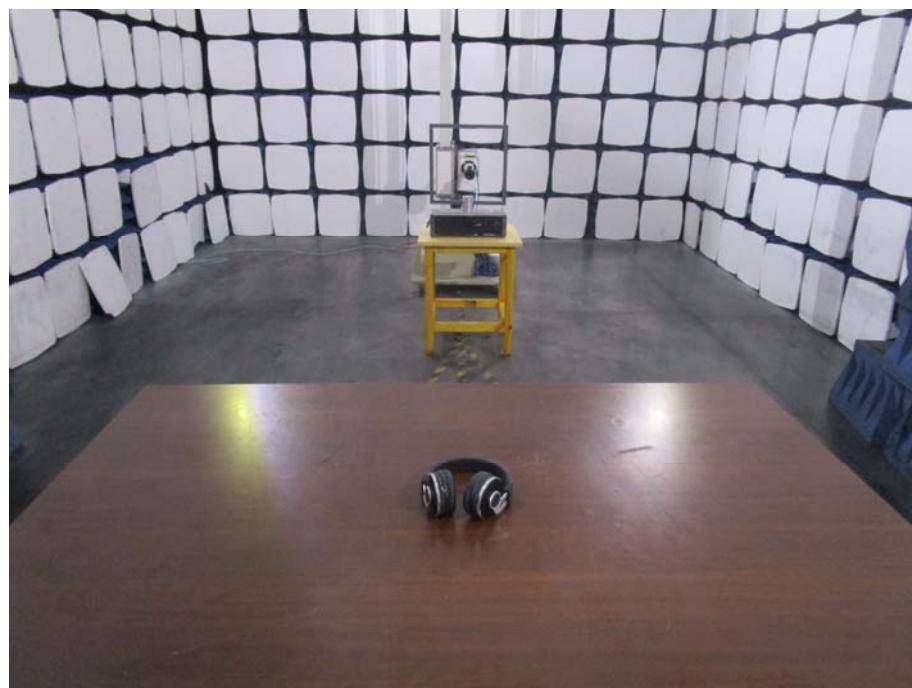
**Radiation Emission Test Setup (30MHz to 1GHz)**
