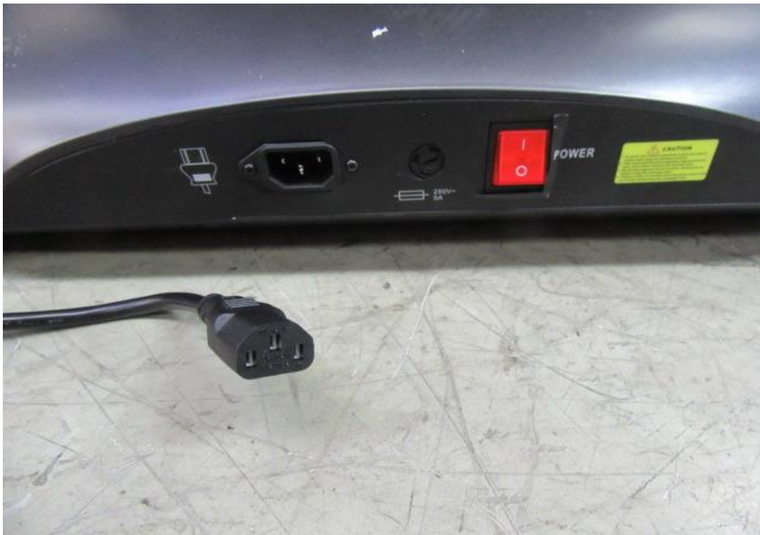
Photo 6 -Cord connector, main Switch, Fuse and appliance inlet
