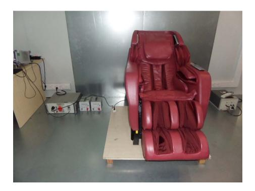
Radiation Emission Test Setup (Below 30MHz)
