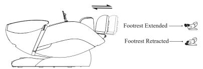
A footrest sensor is set at the bottom of footrest, the footrest will adjust the length automatically once the chair started.
