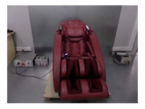
Radiation Emission Test Setup (Below 30MHz)
