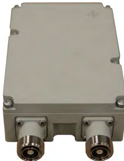
Figure 2-39 LBD Transmit Output Filter (Dielectric Resonator)
