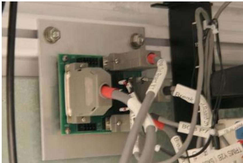
Figure 3-35 Break Out Board Installed in DRU
