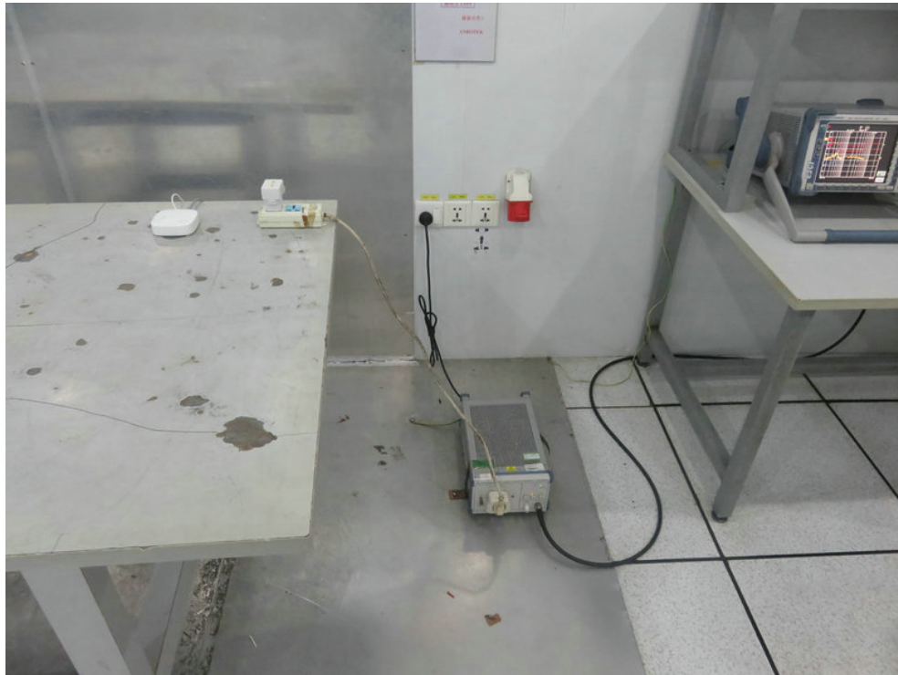
Photo of Conducted Emission Measurement
