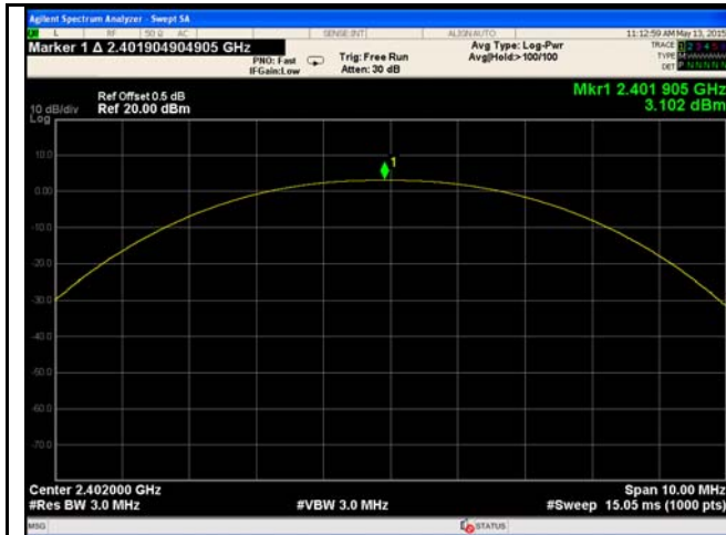
GFSK Output power - Low CH 2402
