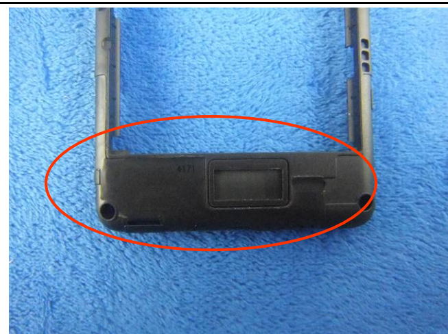
GSM/PCS/UMTS-FDD Antenna View
