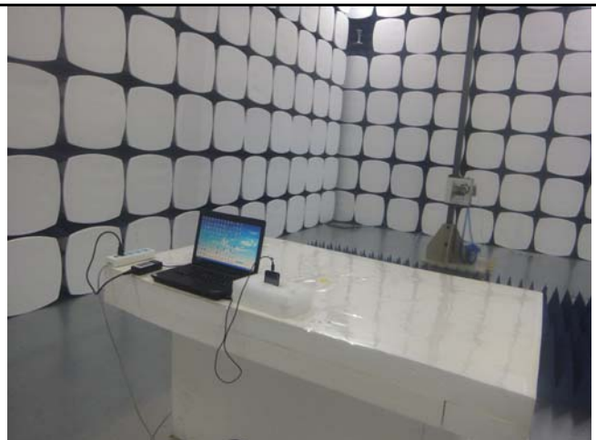
Radiated Spurious Emissions Test Setup Above 1GHz
