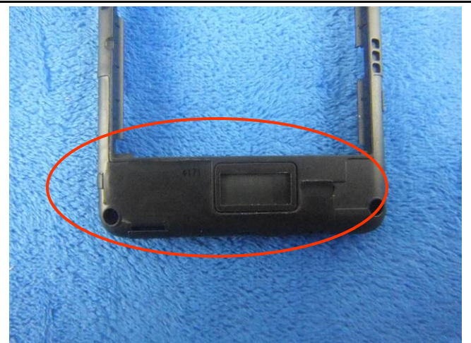
GSM/PCS/UMTS-FDD Antenna View
