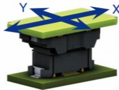
Figure 4: FX23/FX23L XY-Floating Ability
