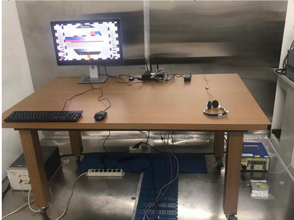
Photograph –Conduction Emission Test Setup
