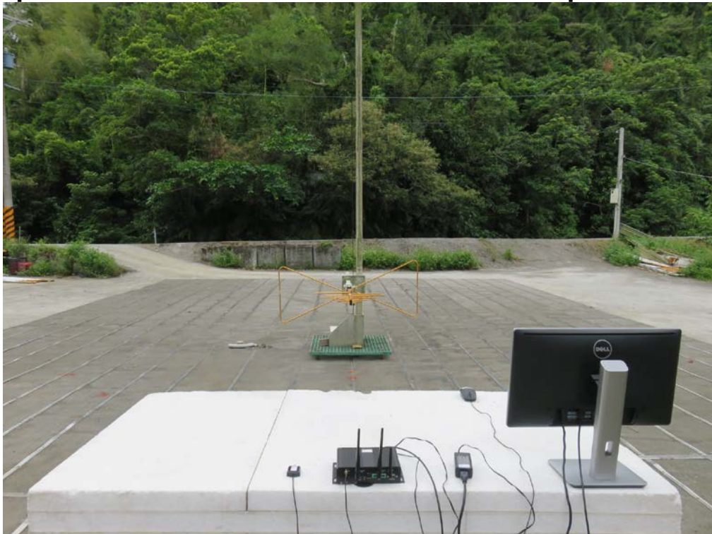
Photograph – Radiated Emission 1G Below Test Setup
