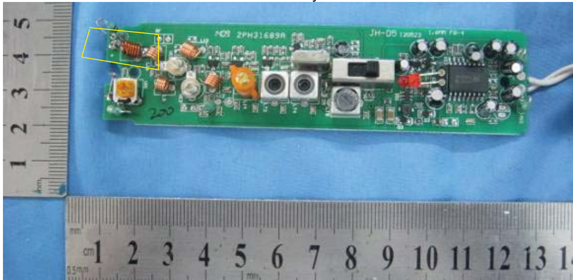
WM-300 with PCB Layout's Antenna
