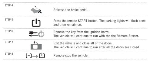
The engine will continue to run until either the remote stop function is pressed (see USING THE RE-MOTE CONTROL, page 5), the Remote-Starter runtime expires, the parking brake is disengaged, the brake is pressed, or the hood is opened. If the Remote-Starter is shut down by transmitter it will automatically go in to Ready Mode (if all the doors are closed).
