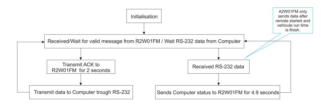
Note: 2ACKU-A2W01FM is powered on 12V DC car battery
