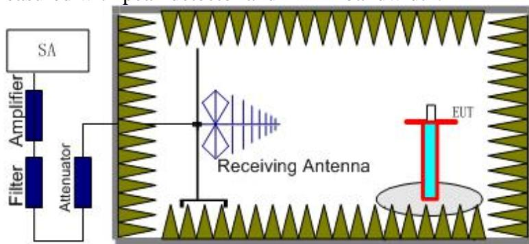
Radiated emissions measurements were made only at the upper, middle, and lower carrier frequencies of the PCS 1900 band (1850.2 MHz, 1880 MHz and 1909.8 MHz) ,GSM850 band (824.2MHz, 836.6MHz, 848.8MHz), UMTS band V(826.4MHz, 835.0MHz, 846.6MHz) . It was decided that measurements at these three carrier frequencies would be sufficient to demonstrate compliance with emissions limits because it was seen that all the significant spurs
