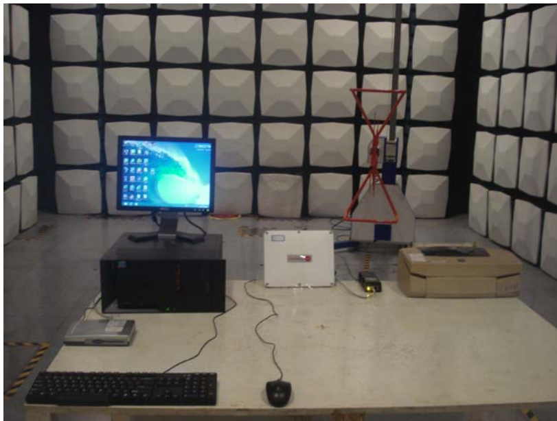
Radiated Emissions Front View (Below 1GHz)
