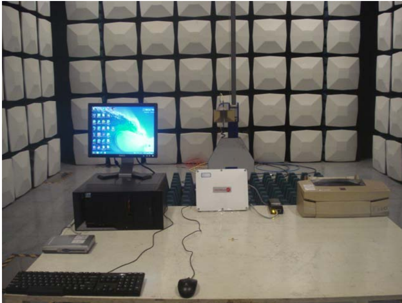
Radiated Emissions Front View (Above 1GHz)
