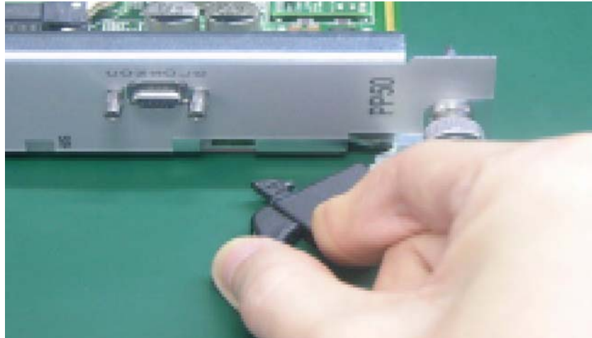
Figure 3-9: Opening the Latch Handle, Lever Release
