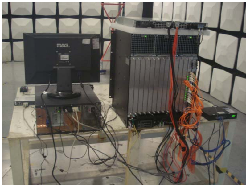
Radiated Disturbance Test Setup (Below 1GHz) Rear View
