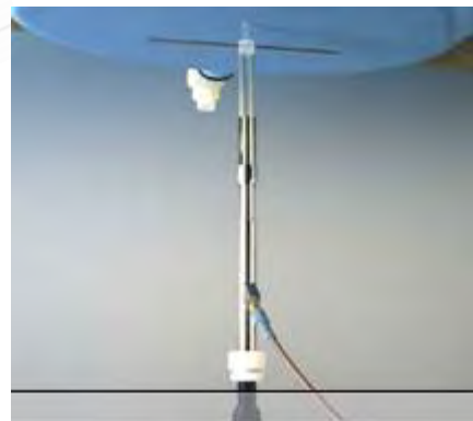
Photograph of the dipole Antenna
