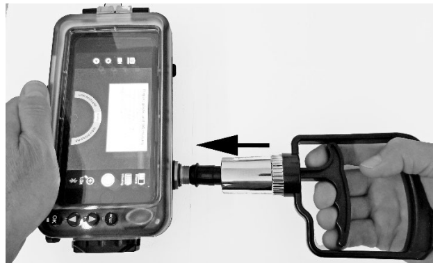
Hand pump pressed against vacuum check port
