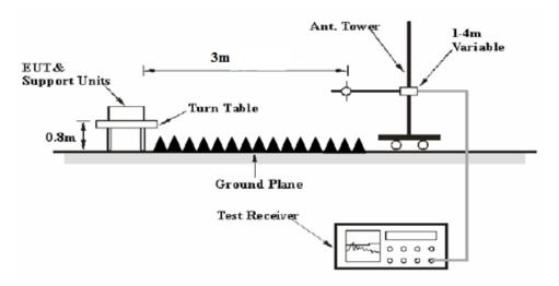
The radiated emission tests were performed in the 3 meters chamber, using the setup accordance with the ANSI C63.4-2003. The specification used was the FCC 15.209 and FCC 15.407 limits.
