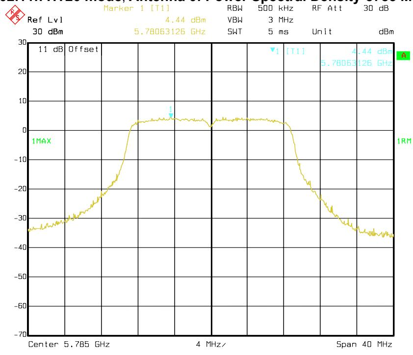
**802.11n HT20 mode, Antenna 0: Power Spectral Density-5825 MHz**
