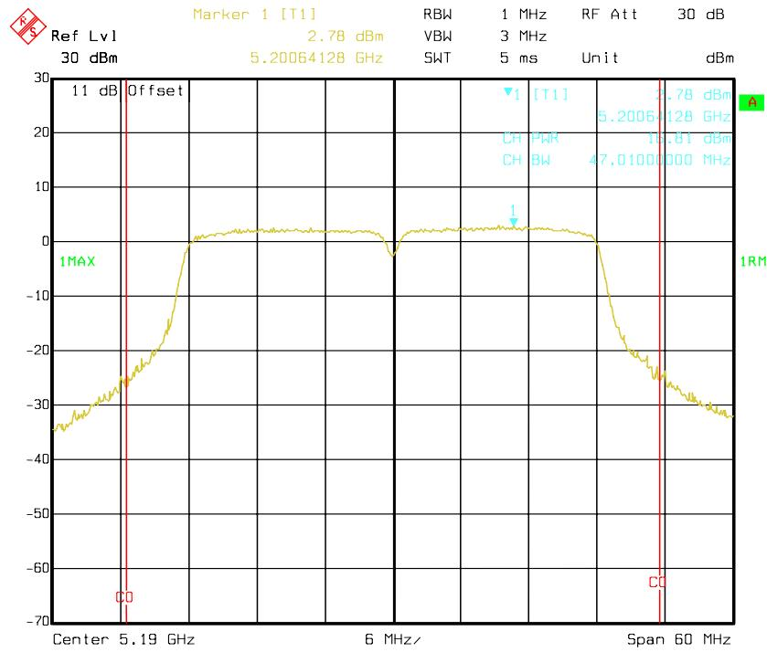
**802.11n HT40 mode, Antenna 0: RF Output Power-5230 MHz**
