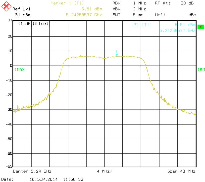
**802.11n HT40 mode, Antenna 0: Power Spectral Density-5190 MHz**
