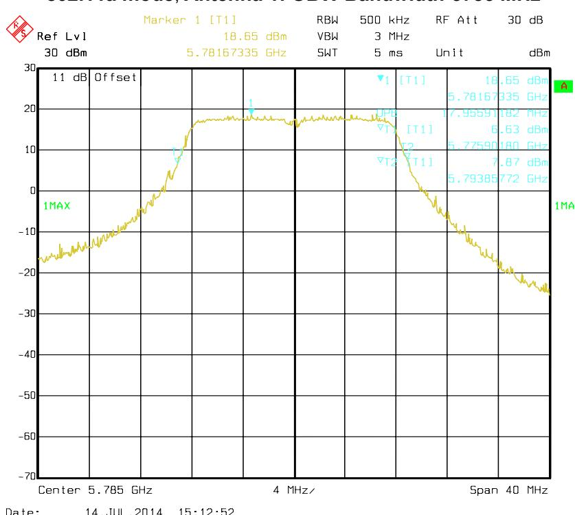
**802.11a mode, Antenna 1: 6 dB Bandwidth-5825 MHz**
