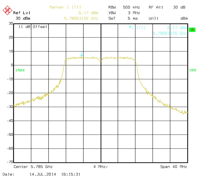
**802.11a mode, Antenna 1: Power Spectral Density-5825 MHz**
