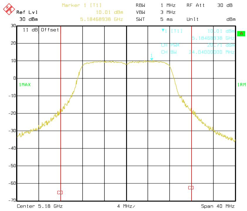
**802.11a, Antenna 1: RF Output Power-5200 MHz**
