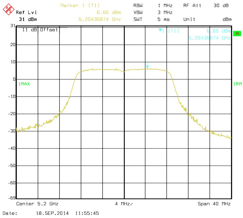
**802.11n HT20 mode, Antenna 0: Power Spectral Density-5240 MHz**
