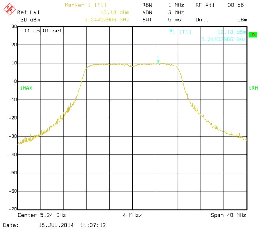
**802.11n HT20 mode, Antenna 0: Power Spectral Density-5180 MHz**
