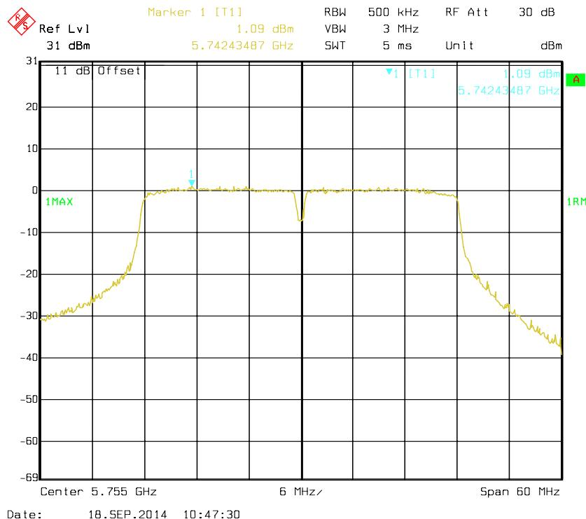
**802.11n HT40 mode, Antenna 1: Power Spectral Density-5795 MHz**
