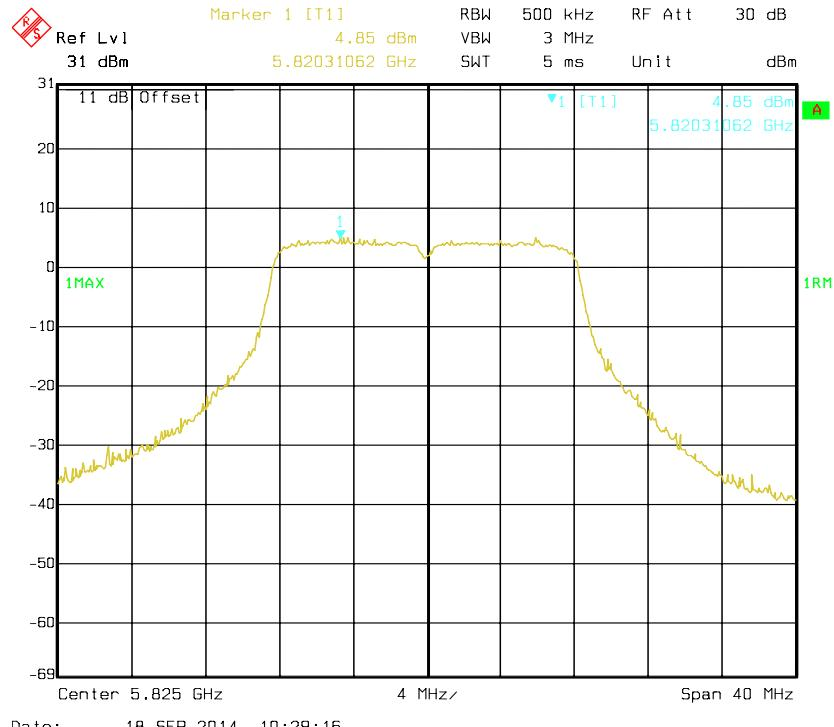
**802.11n HT20 mode, Antenna 0: Power Spectral Density-5745 MHz**
