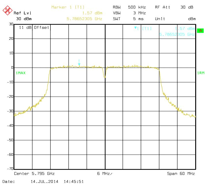
**802.11a mode, Antenna 1: Power Spectral Density-5745 MHz**
