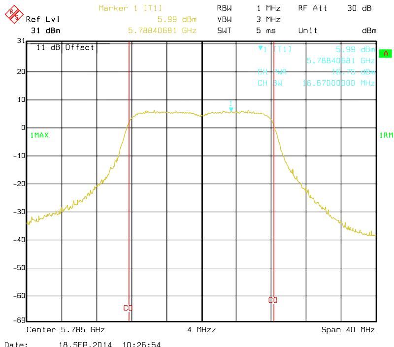
**802.11a, Antenna 0: RF Output Power-5825 MHz**
