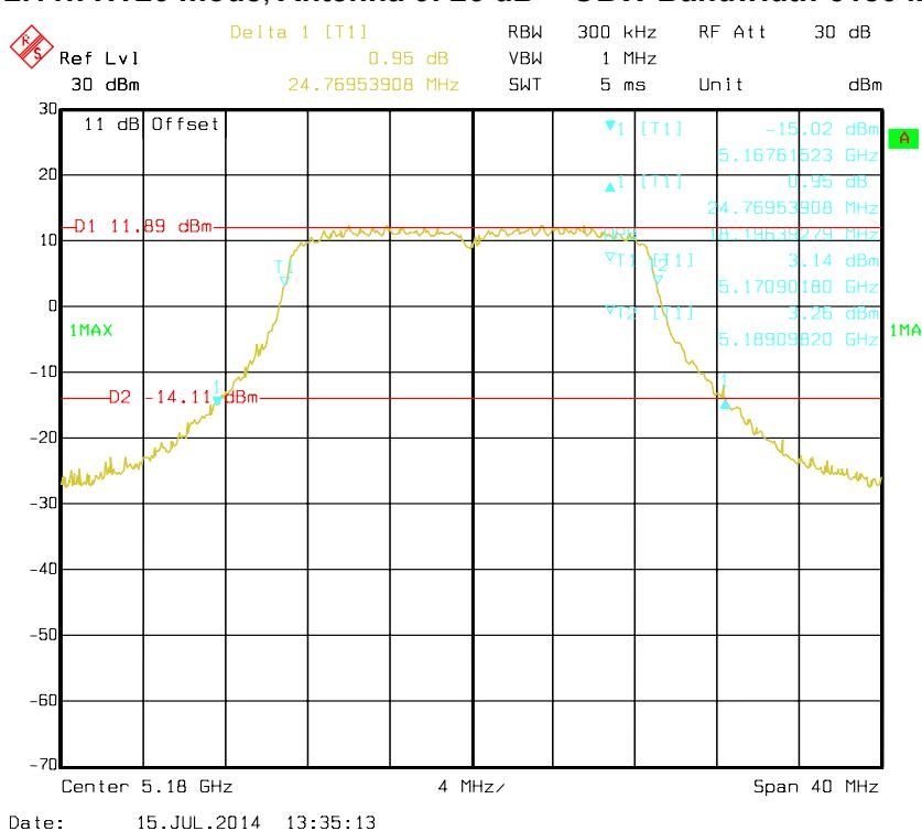
**802.11n HT20 mode, Antenna 0: 26 dB + OBW Bandwidth-5200 MHz**
