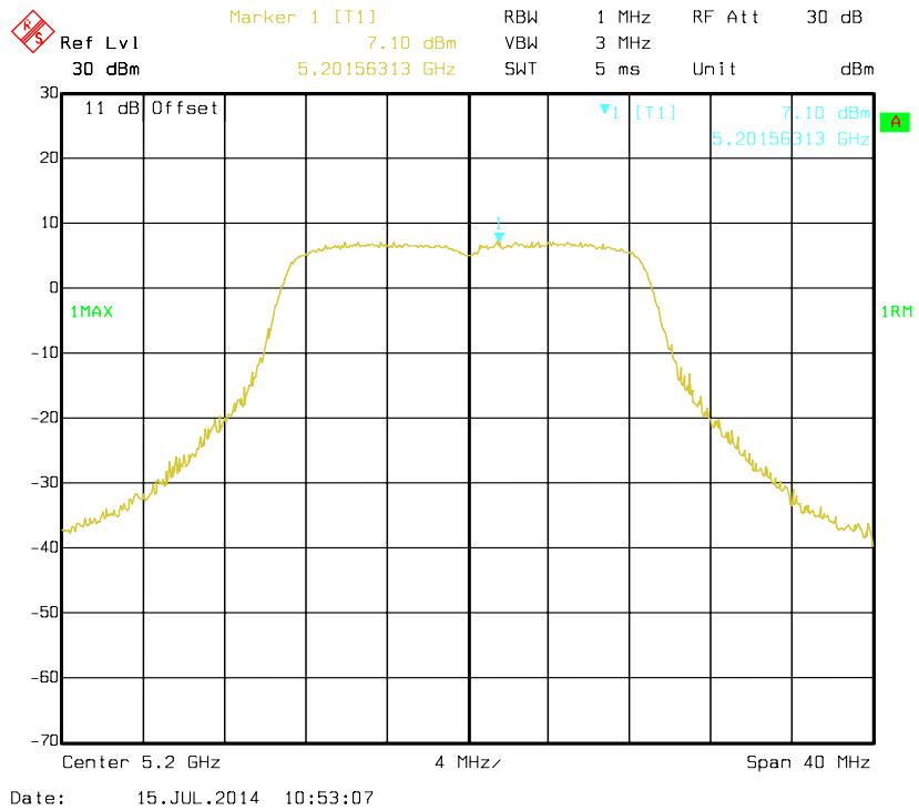
**802.11n HT20 mode, Antenna 1: Power Spectral Density-5240 MHz**
