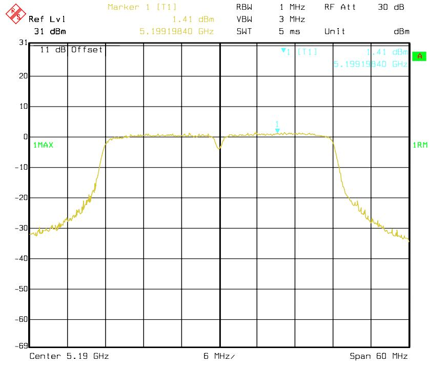
**802.11n HT40 mode, Antenna 0: Power Spectral Density-5230 MHz**
