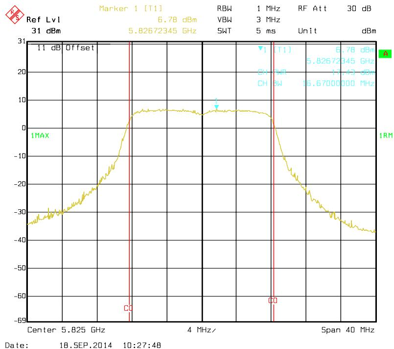
**802.11n HT20 mode, Antenna 0: RF Output Power-5745 MHz**
