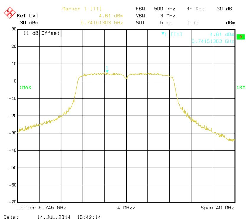
**802.11n HT20 mode, Antenna 1: Power Spectral Density-5785 MHz**
