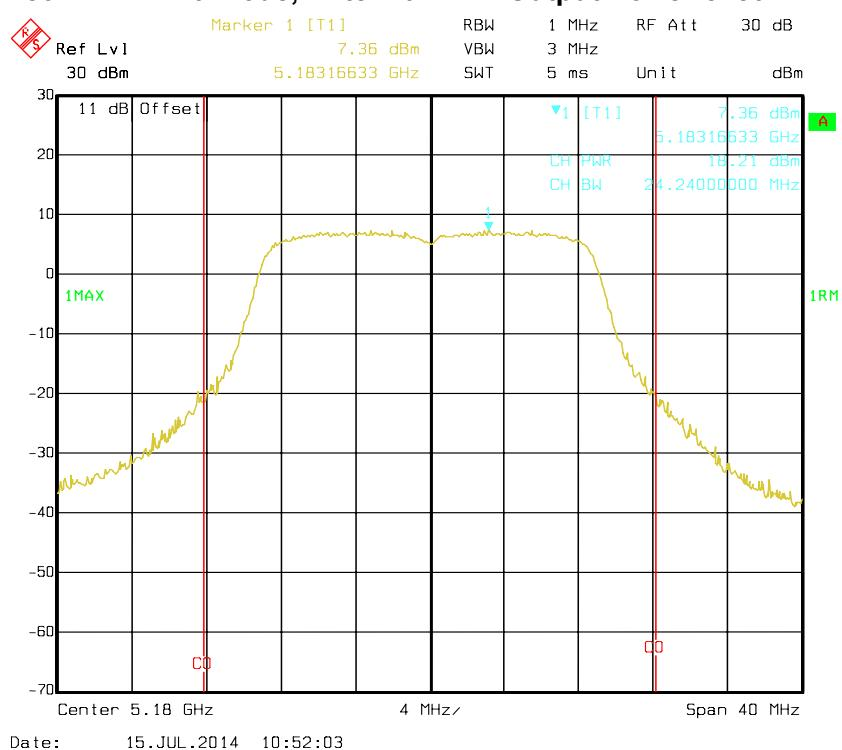
**802.11n HT20 mode, Antenna 1: RF Output Power-5200 MHz**
