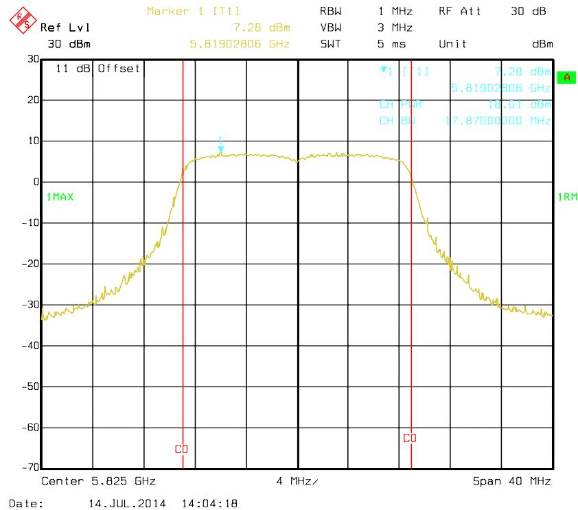
**802.11n HT40 mode, Antenna 0: RF Output Power-5755 MHz**
