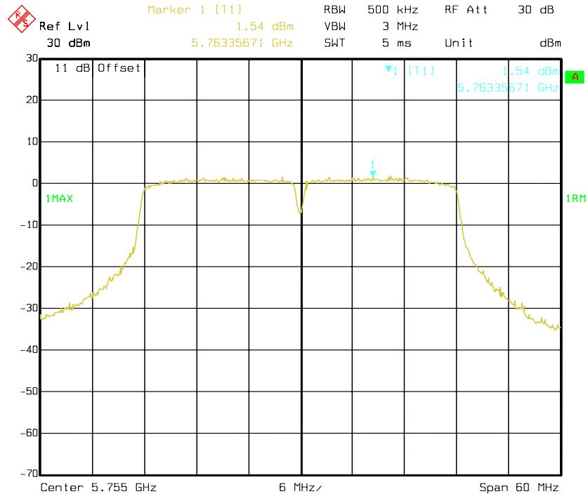
**802.11n HT40 mode, Antenna 0: Power Spectral Density-5795 MHz**
