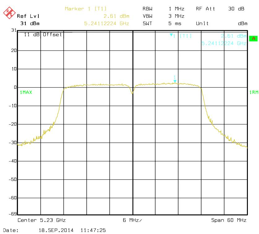
**802.11a mode, Antenna 1: Power Spectral Density-5180 MHz**
