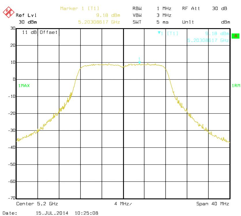
**802.11a mode, Antenna 1: Power Spectral Density-5240 MHz**
