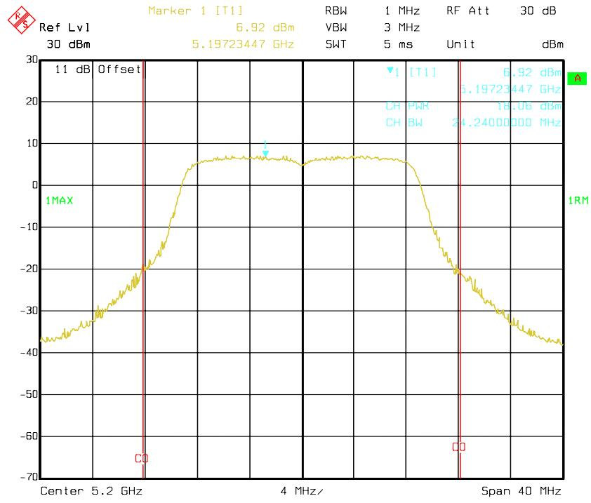
**802.11n HT20 mode, Antenna 1: RF Output Power-5240 MHz**
