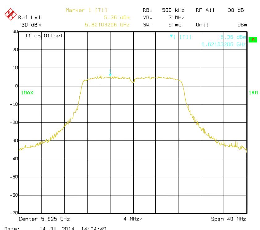
**802.11n HT40 mode, Antenna 0: Power Spectral Density-5755 MHz**
