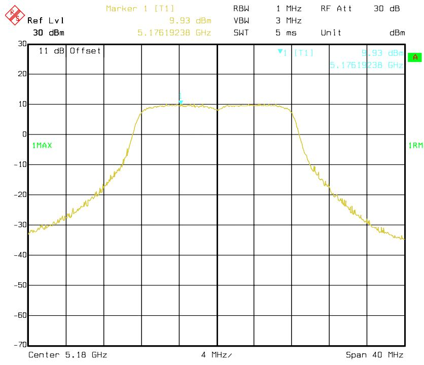
**802.11a mode, Antenna 1: Power Spectral Density-5200 MHz**
