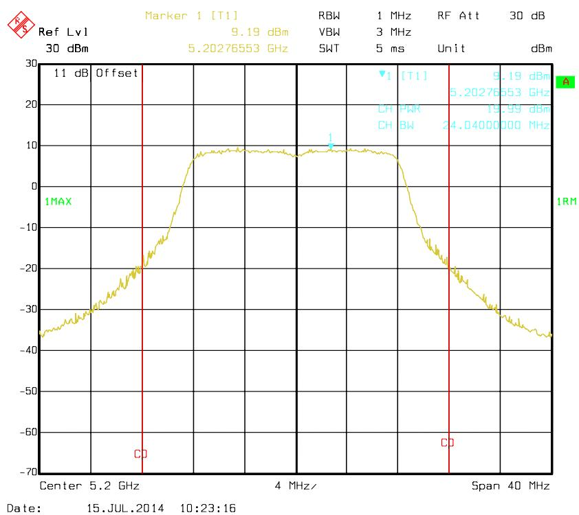
**802.11a, Antenna 1: RF Output Power-5240 MHz**
