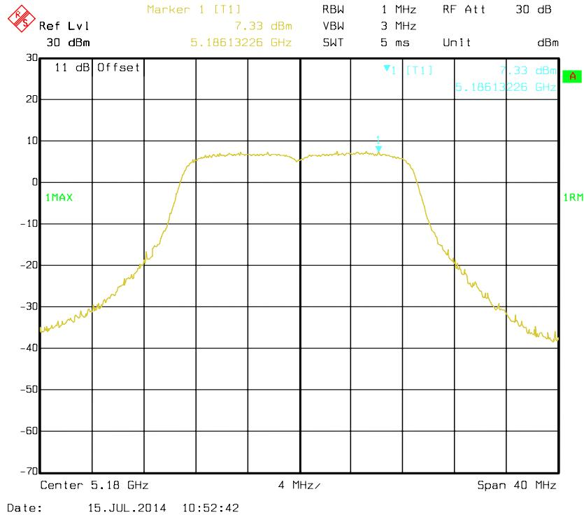
**802.11n HT20 mode, Antenna 1: Power Spectral Density-5200 MHz**
