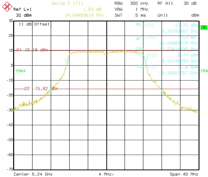
**802.11n HT20 mode, Antenna 0: 26 dB + OBW Bandwidth-5180 MHz**
