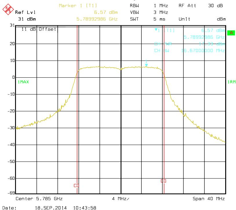
**802.11a, Antenna 1: RF Output Power-5825 MHz**
