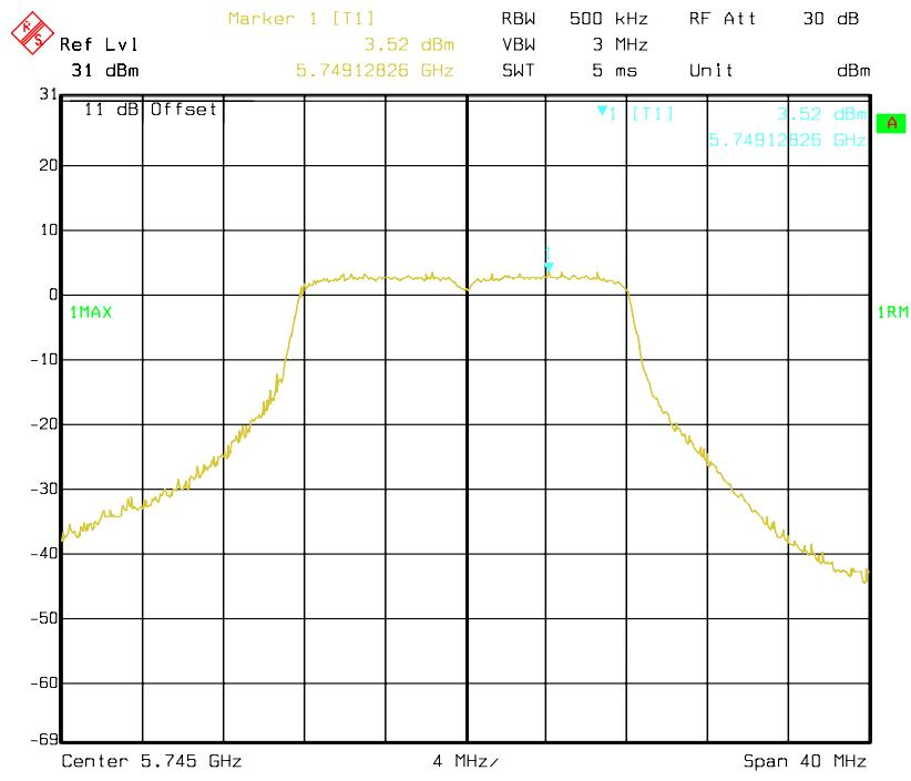
**802.11a mode, Antenna 0: Power Spectral Density-5785 MHz**
