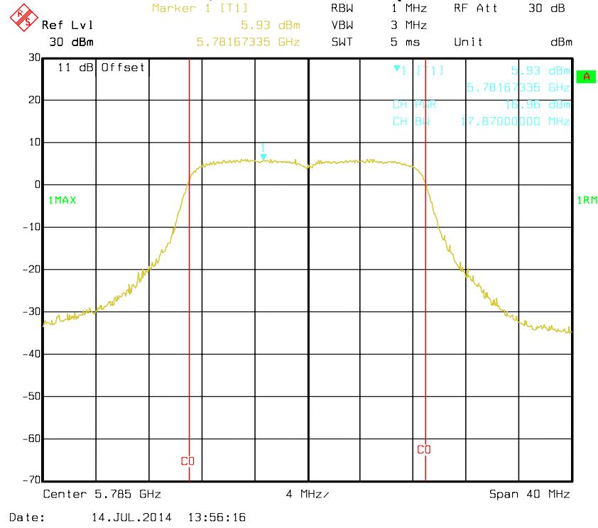
**802.11n HT20 mode, Antenna 0: RF Output Power-5825 MHz**
