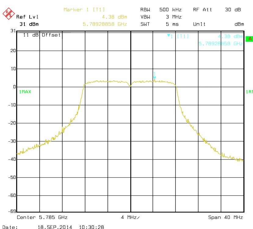
**802.11a mode, Antenna 0: Power Spectral Density-5825 MHz**
