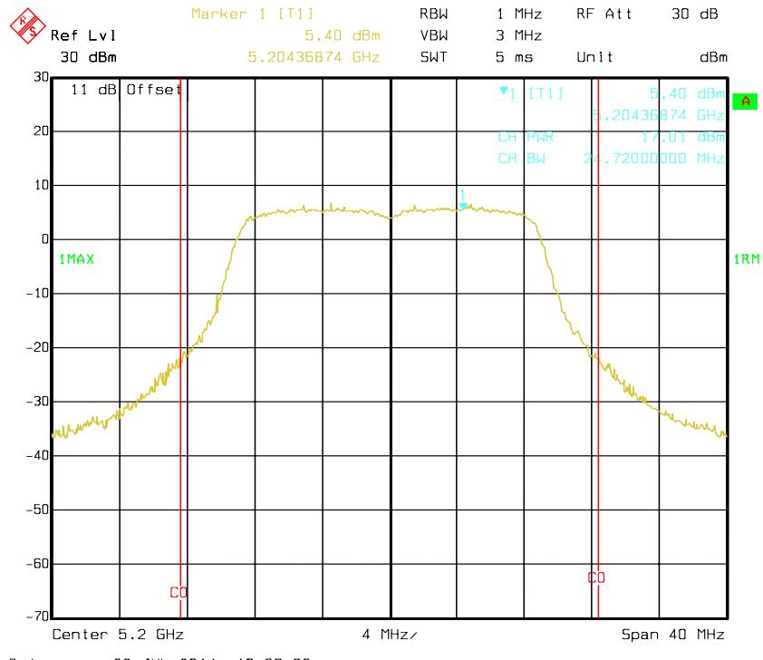
**802.11n HT20 mode, Antenna 0: RF Output Power-5240 MHz**
