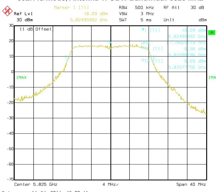
**802.11n HT20 mode, Antenna 1: 6 dB Bandwidth-5745 MHz**
