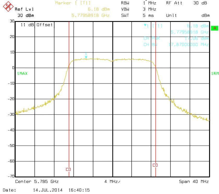
**802.11n HT20 mode, Antenna 1: RF Output Power-5825 MHz**
