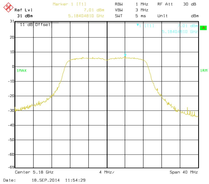
**802.11n HT20 mode, Antenna 0: Power Spectral Density-5200 MHz**
