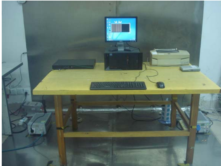
Conducted Emissions Test Setup – Front View
