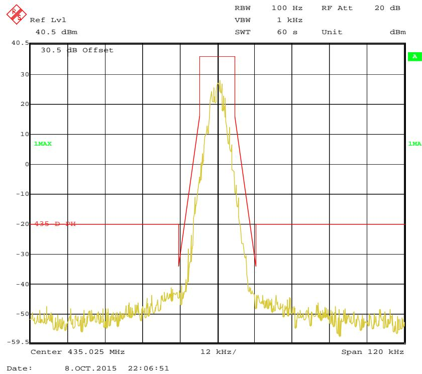
**Emission Mask D with Low Power 12.5 kHz, 435.025 MHz**
