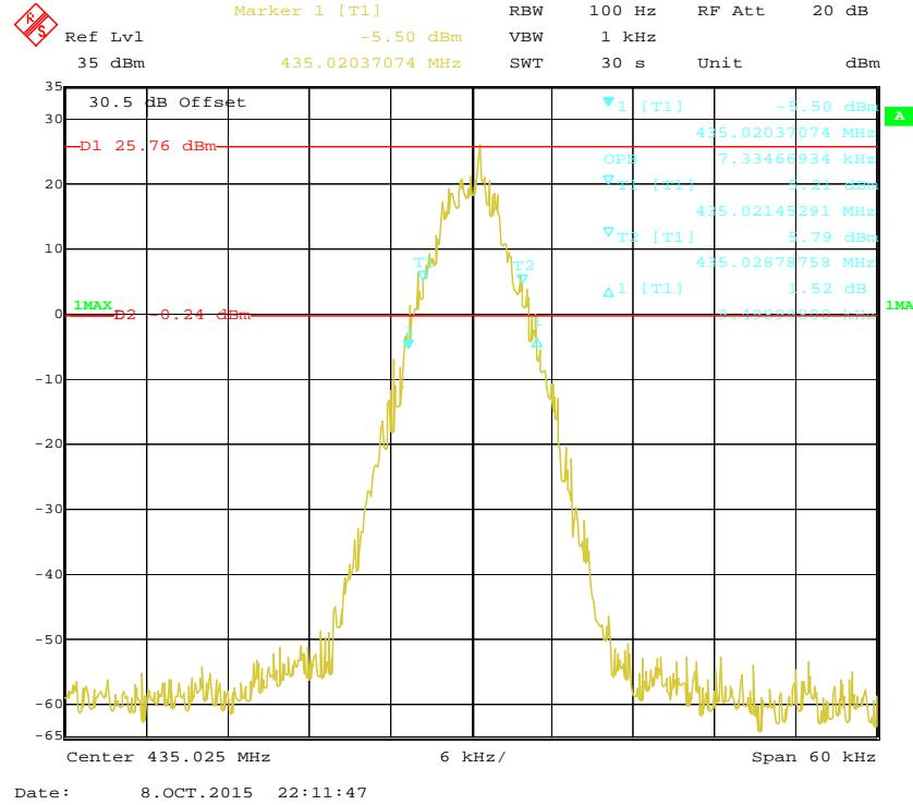
**Emission Mask D with High Power 12.5 kHz, 435.025 MHz**
