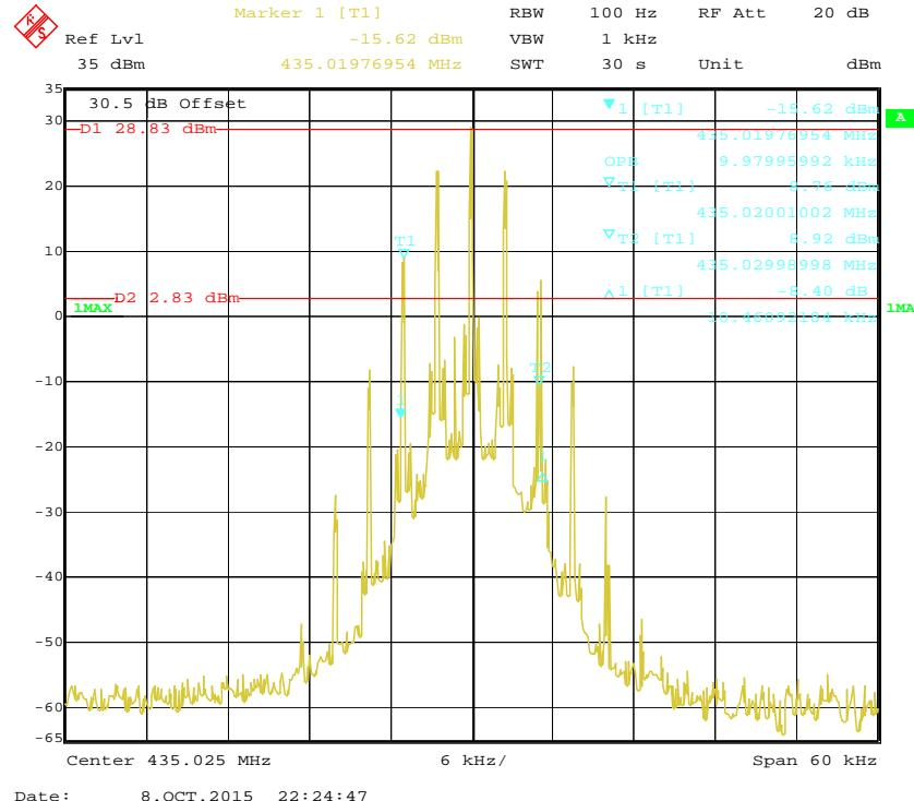
**Emission Mask D with High Power 12.5 kHz, 435.025 MHz**
