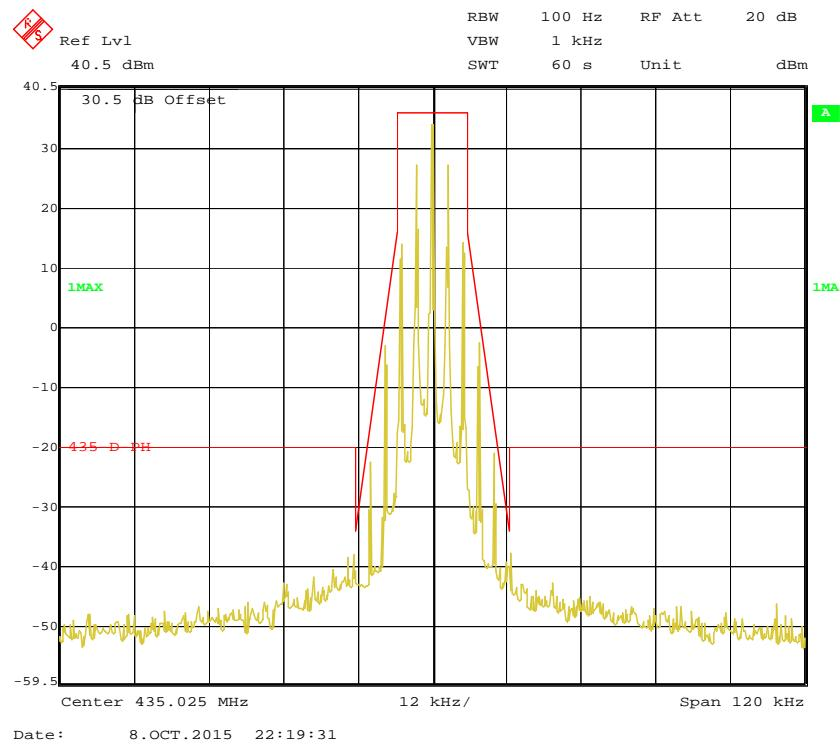
**Emission Mask D with Low Power 12.5 kHz, 435.025 MHz**
