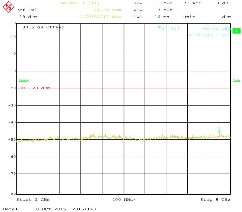
**Digital Modulation:****30 MHz – 1 GHz, Spacing Channel 12.5 kHz, 435.025 MHz**Fund.test with
