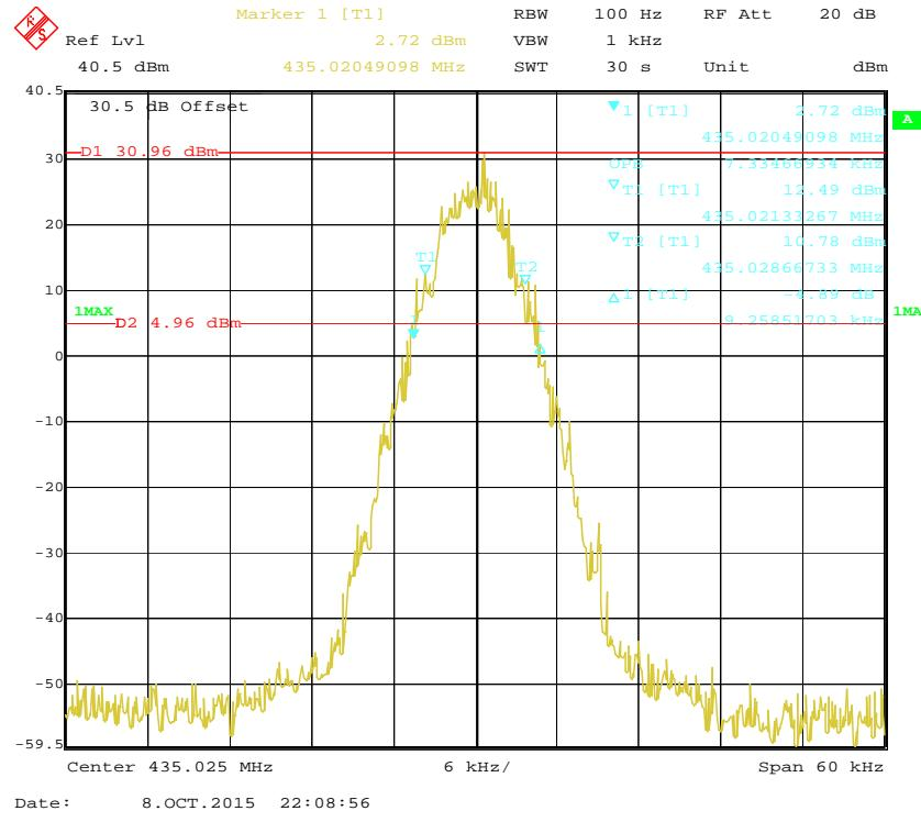
**99% Occupied Bandwidth & 26 dB Emissions Bandwidth 12.5 kHz, 435.025 MHz (Low Power)**
