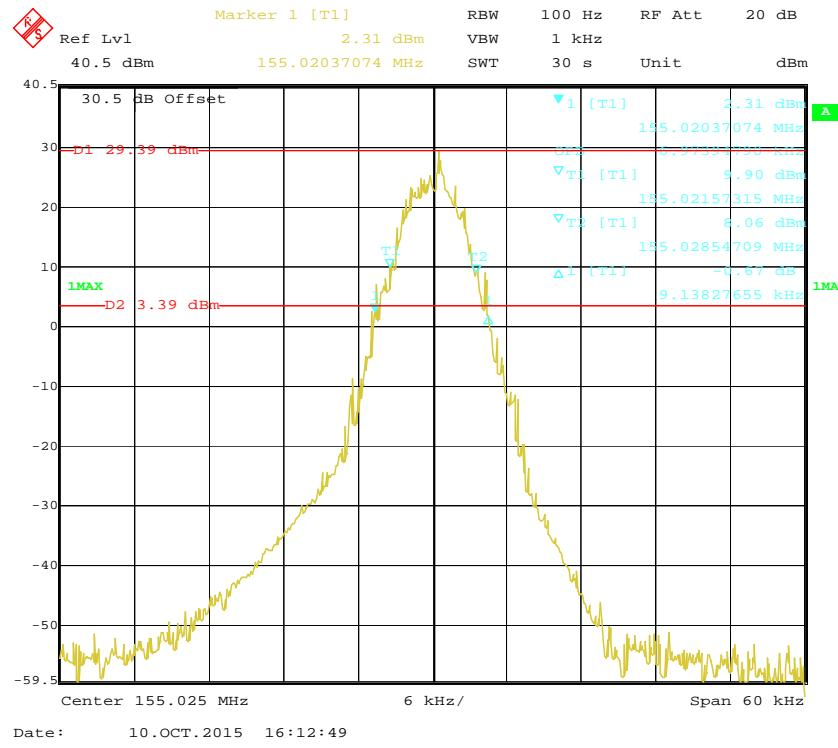
**99% Occupied Bandwidth & 26 dB Emissions Bandwidth 12.5 kHz, 155.025 MHz (Low Power)**
