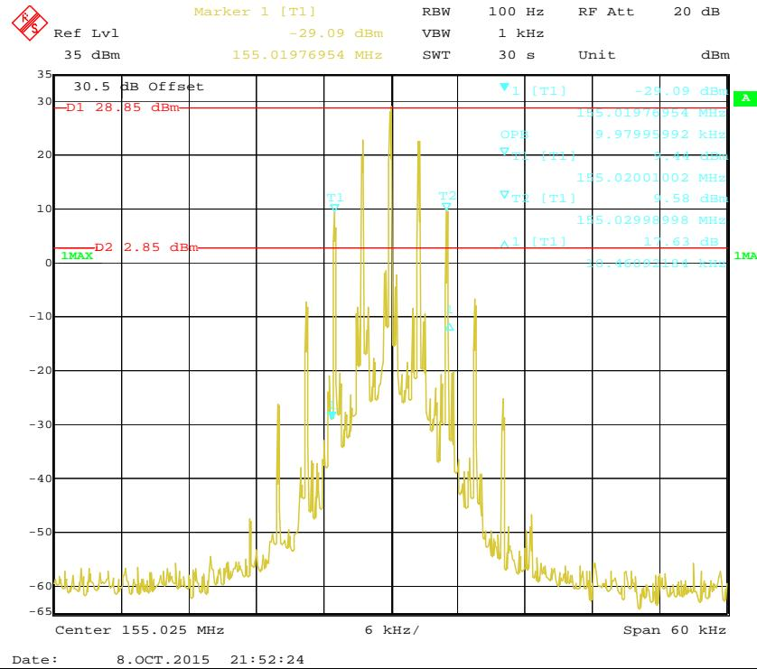
**Emission Mask D with High Power 12.5 kHz, 155.025 MHz**
