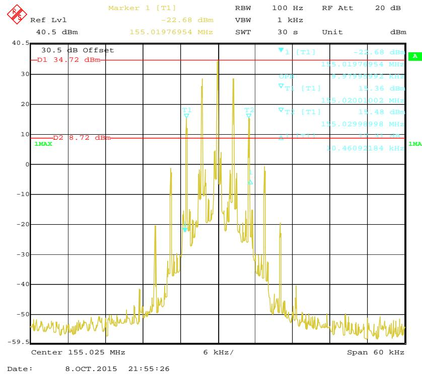
**99% Occupied Bandwidth & 26 dB Emissions Bandwidth 12.5 kHz, 155.025 MHz (Low Power)**
