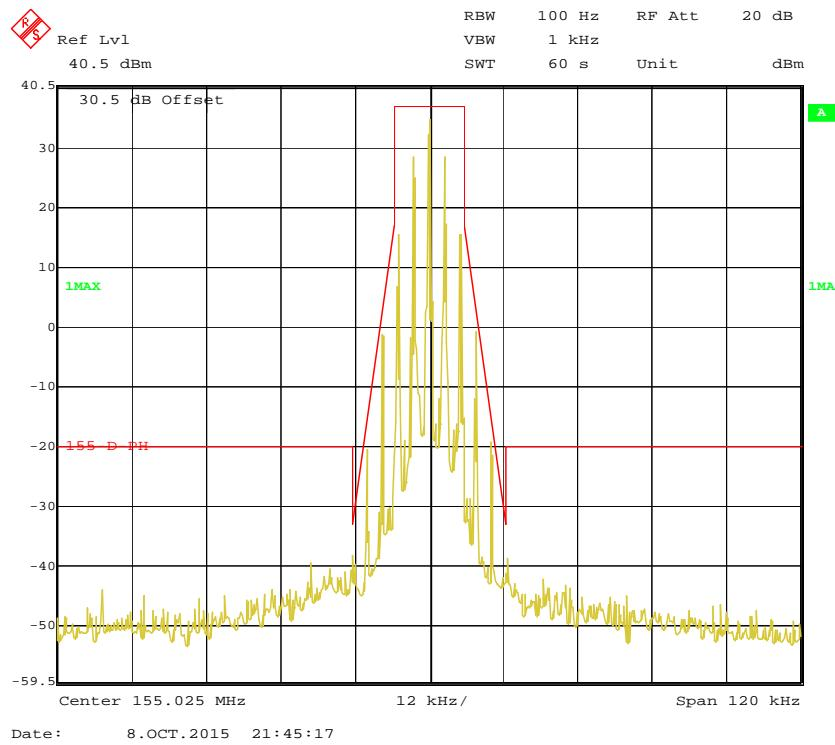
**Emission Mask D with Low Power 12.5 kHz, 155.025 MHz**
