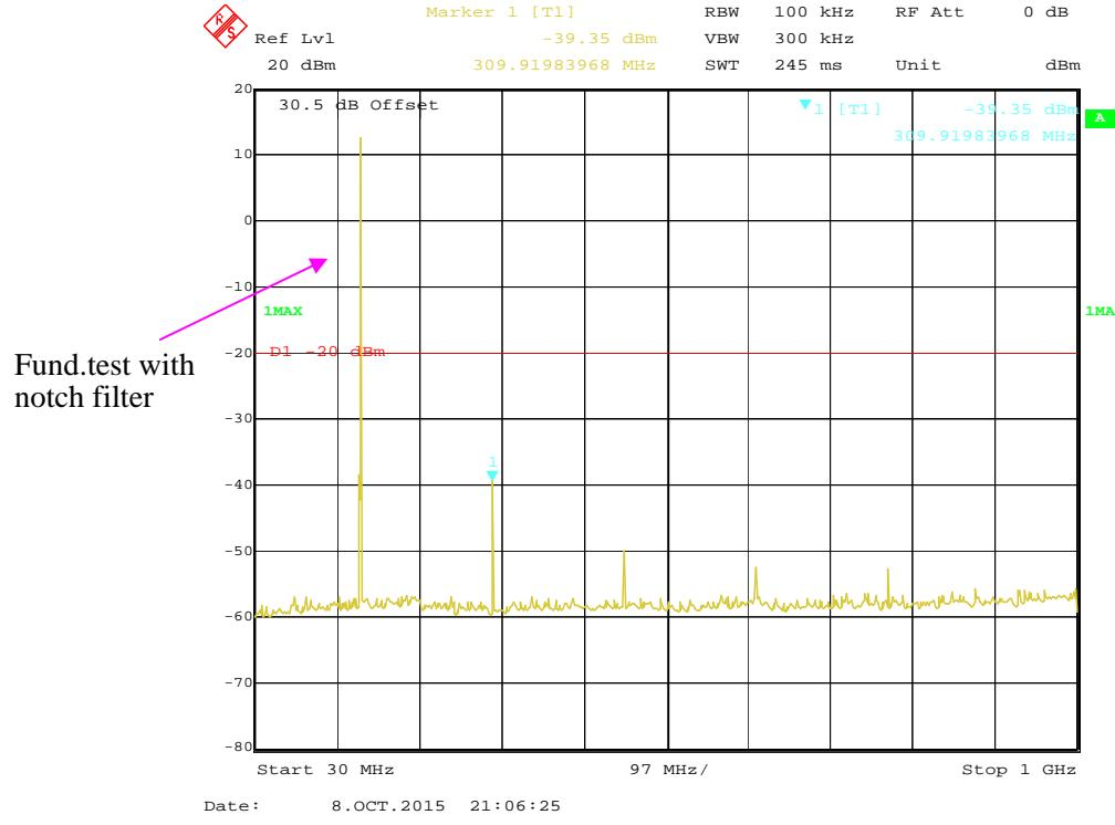
**1 GHz – 2 GHz, Spacing Channel 12.5 kHz, 155.025 MHz**
