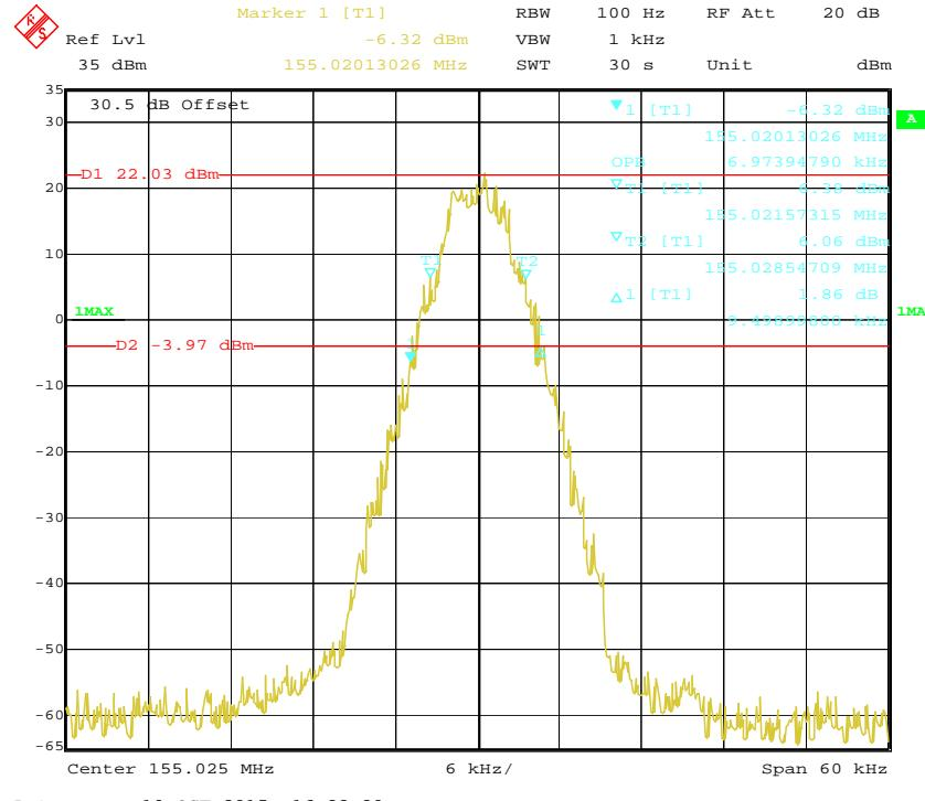
**Emission Mask D with High Power 12.5 kHz, 155.025 MHz**
