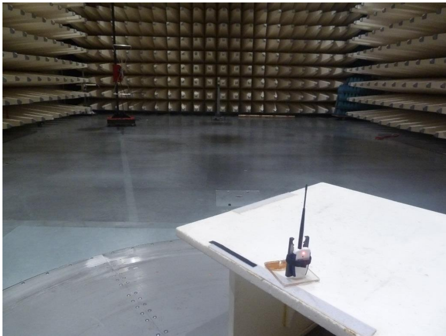
Photo 2: Chamber F – Spurious Emissions radiated 30 MHz – 1 GHz
