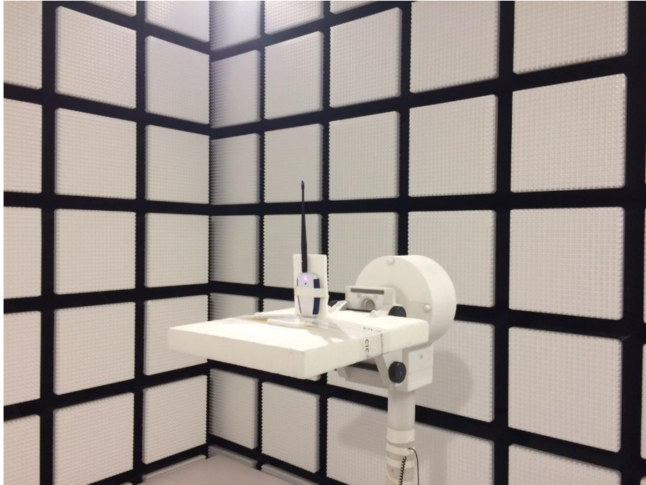
Photo 4: Chamber A – Spurious Emissions radiated 1GHz – 10 GHz
