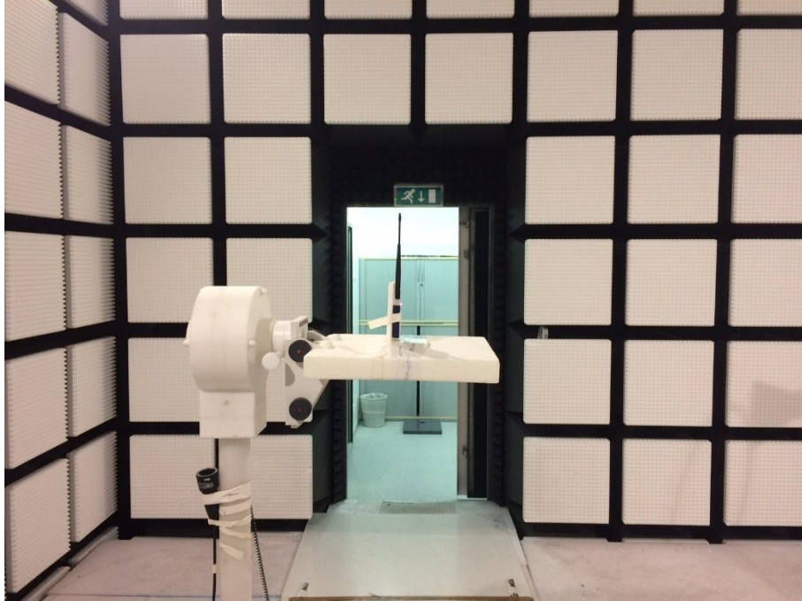
Photo 5: Chamber A – Spurious Emissions radiated 1GHz – 10 GHz
