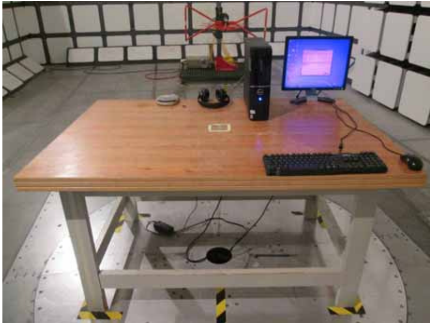
Radiated Emissions – Front View (Below 1 GHz)
