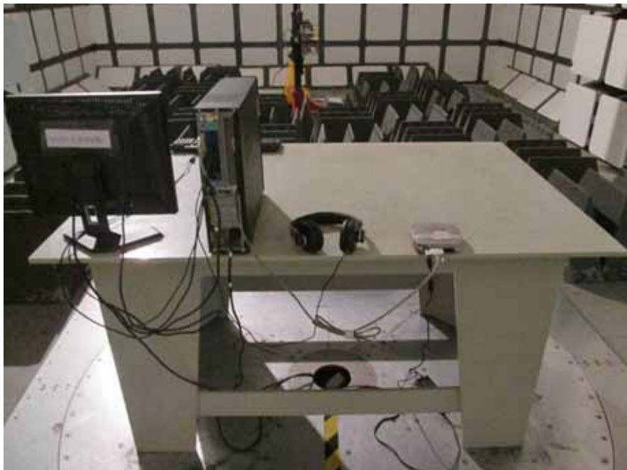
Radiated Emissions – Rear View (Above 1 GHz)
