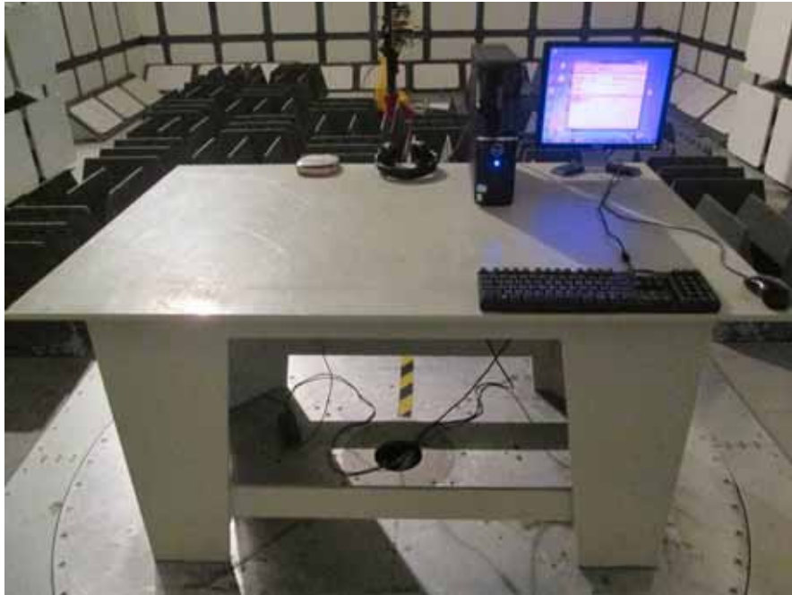
Radiated Emissions – Front View (Above 1 GHz)
