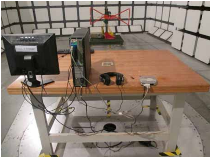
Radiated Emissions – Rear View (Below 1 GHz)
