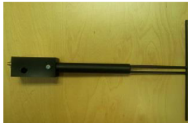
Figure 1 – MVG COMOSAR Validation Dipole
