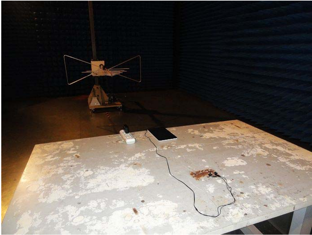
Radiated Emission Test Setup:
