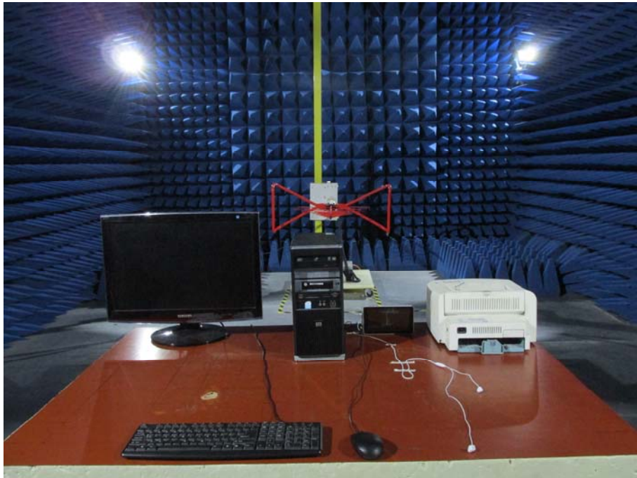
RADIATED EMISSION TEST BELOW 1GHz (Mode 4)
