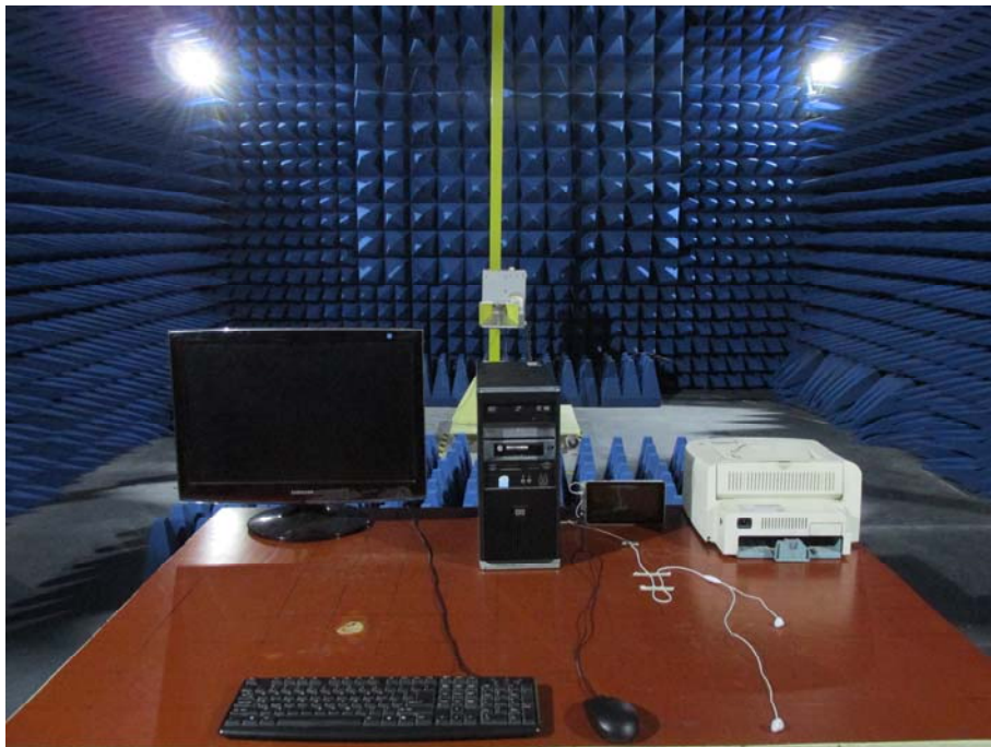
RADIATED EMISSION TEST ABOVE 1GHz (Mode 4)
