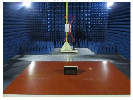
RADIATED EMISSION TEST ABOVE 1GHZ
