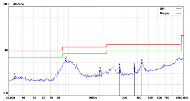
Site Chamber #2 Polarization: Horizontal Temperature: 25 (C)
