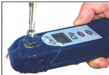
**7** Press **ZERO/ON** and the iDip® display reads 0<sub>PPM</sub> indicating the meter is ready to test. For Standard Liquid Method, place Cell Cover on CELL before zeroing.
