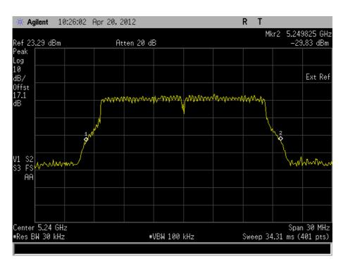
The test was performed on the worst case data rate for 802.11(a) modulation. The worst case was deemed as the data rate which produced the highest level of conducted average power. This data rate was 54Mbps.
