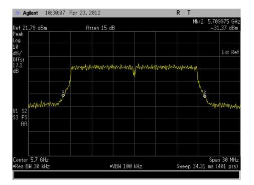
The test was performed on the worst case data rate for 802.11(n) - 20 MHz BW modulation. The worst case was deemed as the data rate which produced the highest level of conducted average power. This data rate was 21.70 Mbps.
