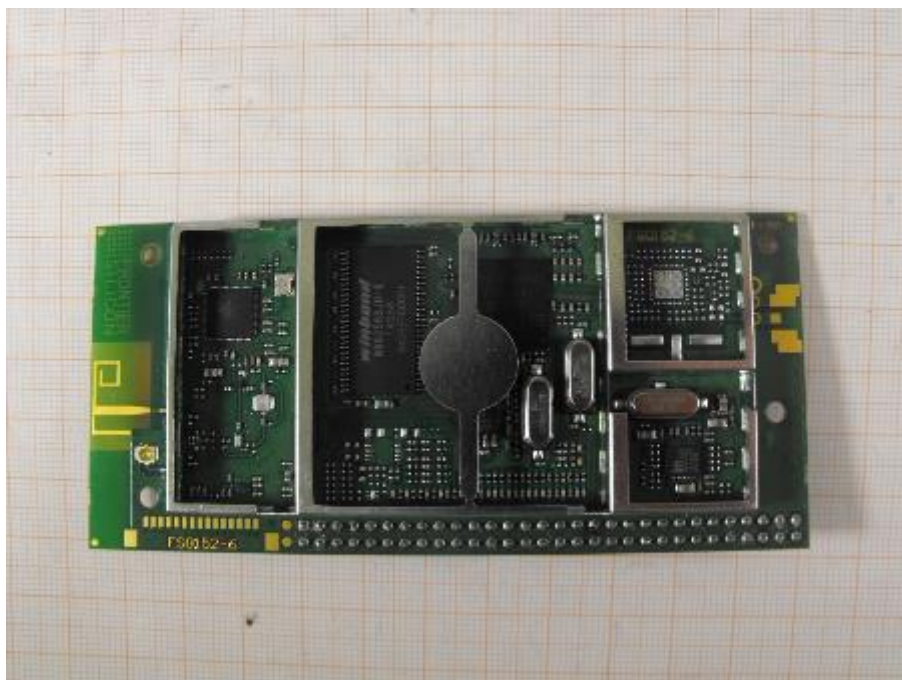
Photo 15: PCB 4 front side without aluminium shielding
