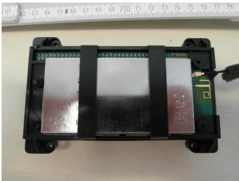
Photo 14: PCB 4 front side with aluminium shielding
