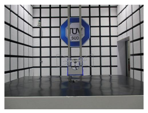
Radiated Emission Test 1GHz-18GHz
