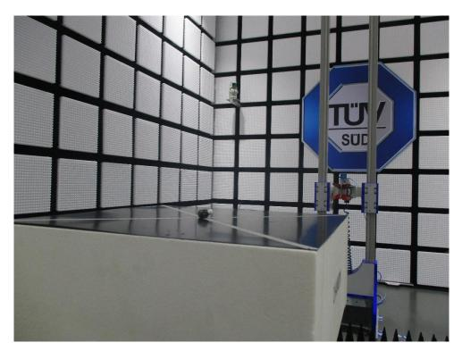
Radiated Emission Test 18GHz-40GHz
