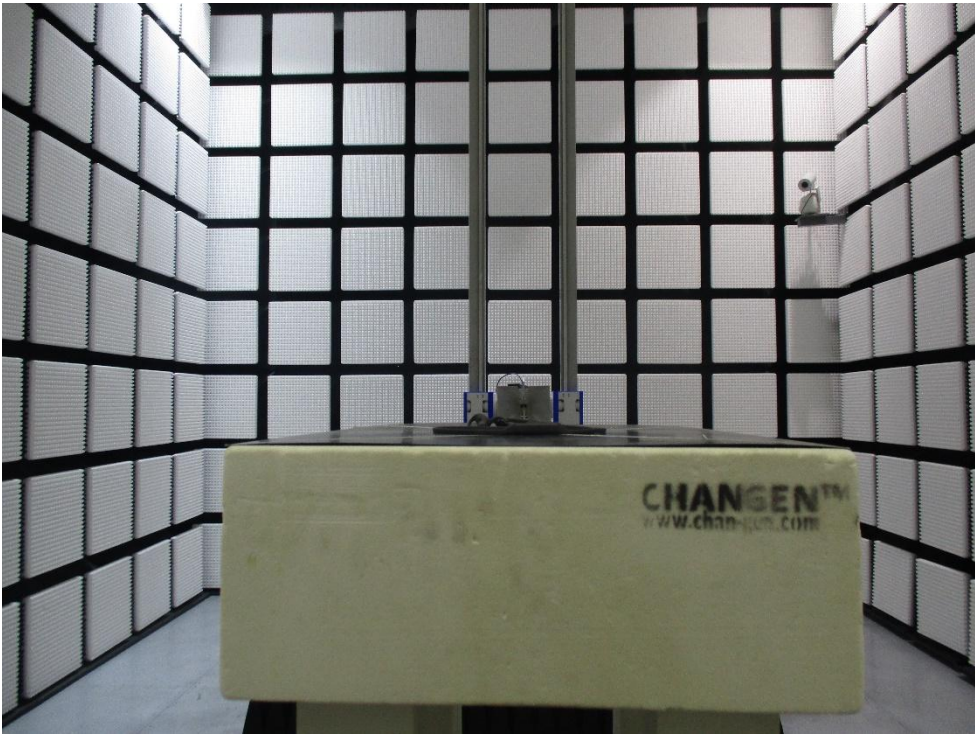
Radiated Emission Test above 1GHz
