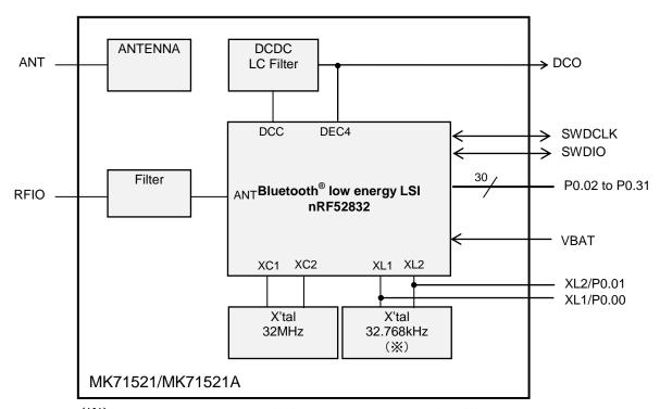
(※) MK71521A does not built-in a 32.768KHz crystal oscillator.
