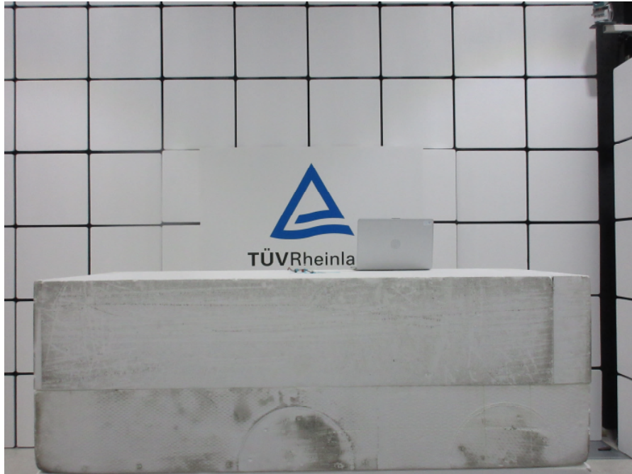
Photograph 1: Set-up for Spurious Emissions (Front View 1)
